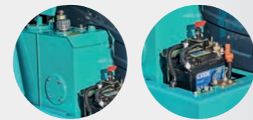
01 FUEL & HYDRAULIC TANK AND BATTERY
